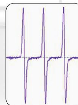
Figure 1: 50 \mu M aqueous TEMPOL in 1 scan, 1 mm capillary Limit of Detection: 40 nM in PBS
