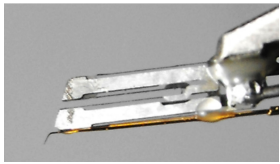
NSOM Probe mounted on tuning fork
