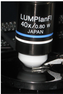
Online integration with Water Immersion Objectives from above for Liquid Cell operation.
