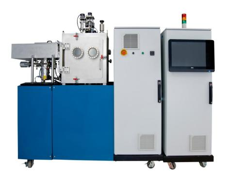
FLEX2000- stand alone multi process chamber tool with deposition up to 2" (2002), 4" (2004) and 8" (2008) round wafers. Multiple and co-depositions up to six sources using either sputtering or thermal evaporation , substrate rotation and 400°C substrate temperature standard. State of the art thin film process recipe for various thin films.
