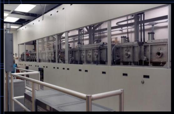
FLEX5000- Inline multi process and multi chambers prototyping production tool, with deposition up to 20" square substrates. Processes include PECVD, HWCVD, ICP and Sputtering. State of the art thin film process recipe for various thin films and devices
