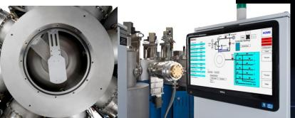
Example of FLEX3008- Six (6) PECVD process zones with a central robotic module for vertical upwards deposition up to 8" (3008) round wafers and 400°C substrate heating capability
