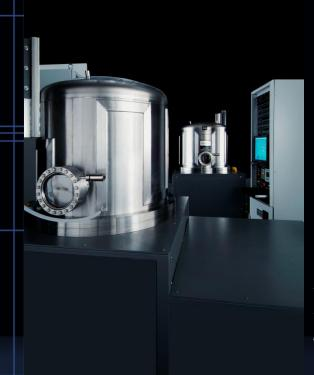
FLEX6000- Roll to roll vertical process tool, with deposition up to 8" (6008) and 14" (6014) wide rolls. Processes include PECVD, HWCVD and Sputtering with a cold drum or 400°C web heating capability. Web materials include, Plastic, metal, Kapton, etc. State of the art thin film process recipe for various thin films.
