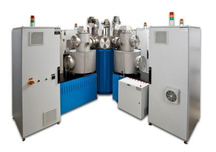
Example of FLEX3004- four (4) PECVD process zones, two (2) multi-source magnetron sputtering zones and a hot wire CVD (HWCVD) zone with a central robotic module for vertical upwards deposition up to 4" (3004) round wafers up to 400°C substrate heating capability
