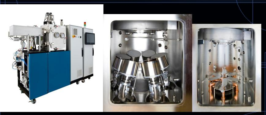
Examples of FLEX2008- Six (6) co-sputtering process zones or six (6) co-thermal process zones for vertical upwards deposition up to 8" round wafers and 800°C substrate temperature.
