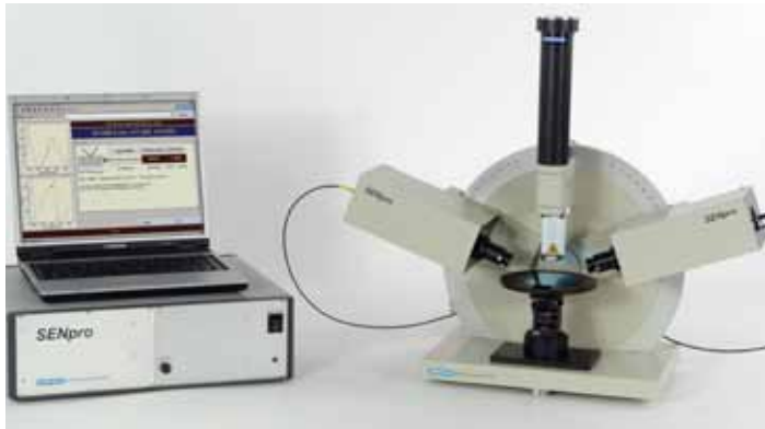
Spectroscopic ellipsometer SENpro with controller and laptop
