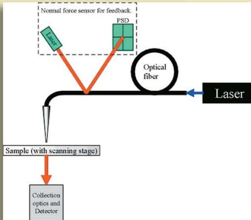
NSOM (SNOM) is the only way to get sub-wavelength optical information from a sample, and as it is usually combined with AFM, the optical information can easily be correlated to topographical information.
