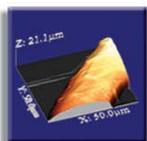
AFM of a wool fiber, that is uniquely imaged with the MV 1000 system which is capable of such imaging as a result of a Z range (100 microns) 5 times larger than any other AFM system.
