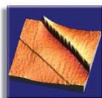
The Nanonics SPMINSOM system integrated with a dual microscope allows for the imaging of a single atomic step of highly oriented pyrolytic graphite as is seen in the lower left of this image.
