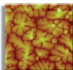
Nanonics SPM/NSOM systems can use any probe and can image with any mode presently known to AFM or NSOM. Seen in this image is a dendritic structure of pentacene imaged with a standard Si cantilevered probe.
