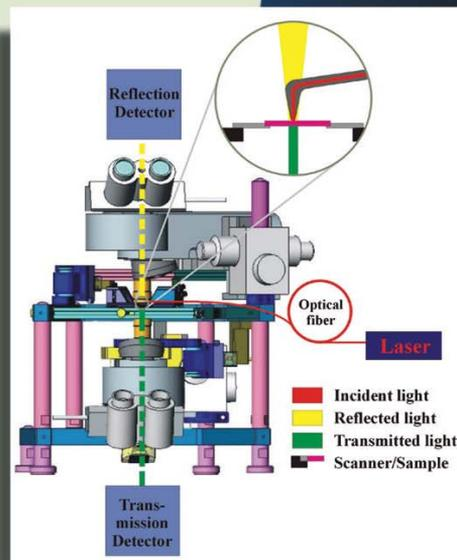
Complete MultiView 1000™ system with a dual microscope providing optics for the collection of transmitted/reflected light and for viewing the sample before and during the AFM scan. The system is also available with either an upright or an inverted microscope. A cantilevered optical fiber is used to illuminate the sample.
