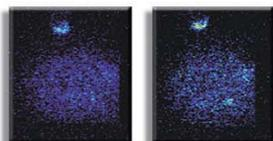
The MV 1000 SPMINSOM system allows for full integration with beam scanning confocal microscopes. Shown is a neuronal cell filled with a calcium sensitive dye that is also held in the tip of an ion sensing glass sensor. The sensor is held above the cellular membrane with AFM control. Images are before (left) and after caffeine activation. *Nature Biotechnology* 21, 1378 (2003)
