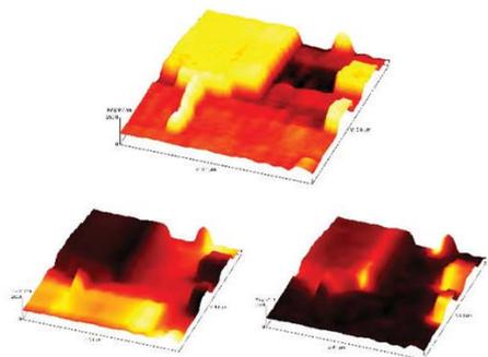
3D AFM topography (top) of a state of the art transistor with on-line pixel by pixel correlation of the Raman spectral distribution of silicon (bottom left) and strained silicon (bottom right). The images represent true chemical distribution since the on-line AFM acts as the finest autofocus mechanism known to date while providing detailed structural correlation.
