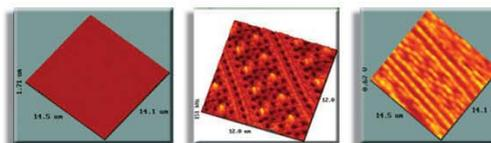
Images of SRAM after chemical mechanical polishing (CMP). The left image shows the AFM of the highly polished surface. The middle image demonstrates excellent reflection NSOM capabilities showing the region underlying the polished surface. The right image displays the superior capabilities of thermal conductivity imaging with Nanonics' specialized probes.
